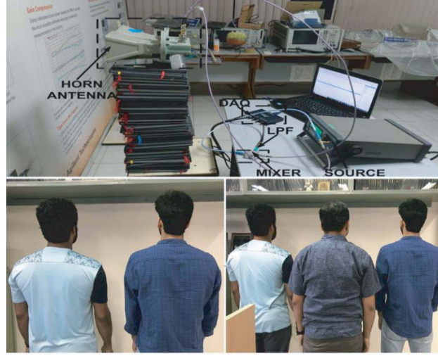
Figure 3. Experimental setup for through the wall measurement of respiration rates.
