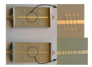
**Figure 14.** Photograph of the fabricated prototypes, 4LH-Π-Spiral at the top and 2LH-T-Stub at the bottom.
