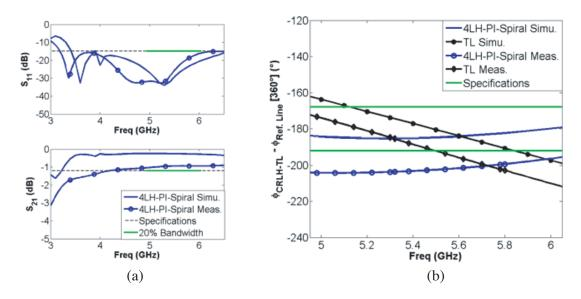
Figure 16. 4LH-PI-Spiral CRLH-TL and simple TL performances in terms of (a)  $S_{11}$ ,  $S_{21}$  and (b) differential phase shift within the BW<sub>T</sub>.
