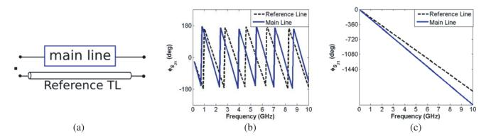
**Figure 1.** (a) Illustration of the concept of DPS, (b) wrapped phase behavior for the reference and main lines of the DPS and (c) unwrapped phase shift behavior of those lines.
