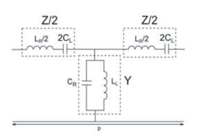
**Figure 4.** Equivalent circuit model for the CRLH TL unit cell.
