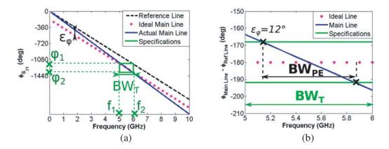
Figure 2. (a) Illustration of the difference in phase between an ideal main line of a DPS and its actual main line for a 180° TL DPS through their unwrapped phase behavior and (b) illustration of the phase error bandwidth  $BW_{PE}$  and targeted bandwidth  $BW_{T}$  for the same DPS with a tolerated phase error of  $\pm 12^{\circ}$ .
