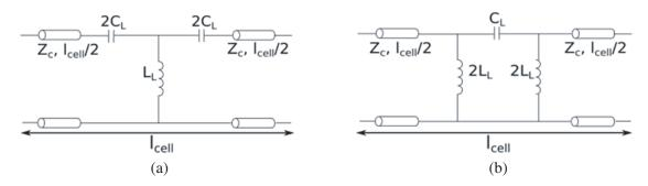
**Figure 8.** Equivalent circuits of a CRLH-TL unit cell: in (a) T-network and (b) Π-network.
