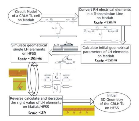
Figure 11. Flowchart of the design method of the 3D geometry of the CRLH-TL from its equivalent circuit model.
