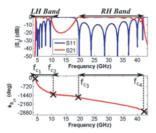
**Figure 5.** Magnitude of  $S_{ij}$  and phase of  $S_{21}$  for the equivalent circuit model of an 8 cells CRLH line.
