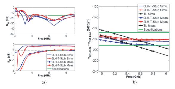
**Figure 15.** 0LH, 2LH-T-Stub CRLH-TLs and simple TL performances in terms of (a)  $S_{11}$ ,  $S_{21}$  and (b) differential phase shift within the BW<sub>T</sub>.
