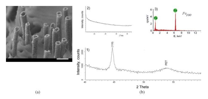
Figure 1. (a) SEM images of the nanostructures under study; (b) X-ray diffractogram of the studied nanostructures: 1) diffractogram in the range of  $2\theta = 40-60^{\circ}$ ; diffractogram in the range of  $2\theta = 20-35^{\circ}$ ; 3) EDA spectrum of the studied nanowires.
