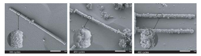
Figure 3. SEM images of the dynamics of changes in the morphology of nanostructures after life tests.
