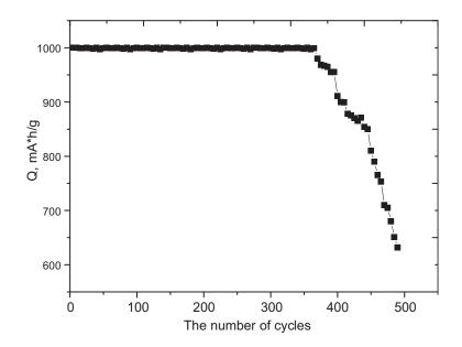
Figure 2. Graph of specific discharge capacity versus the number of cycles tested in charge capacity 1000 mA h/g.
