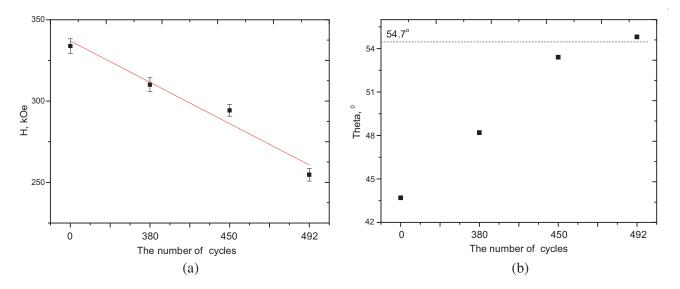
Figure 6. (a) Dynamics of change in the magnitude of the hyperfine magnetic field; Graph of changes in the average value of the angle  $\theta$ . (The line on the graph shows the characteristic value for the absence of ordering of magnetic moments).
