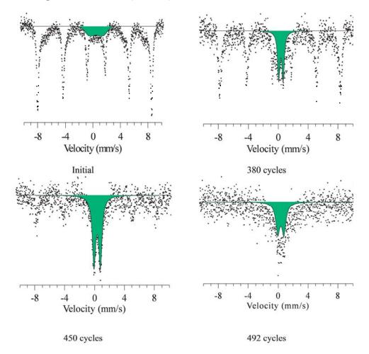
Figure 4. Mossbauer spectra of the studied nanotubes before and after the life test.
