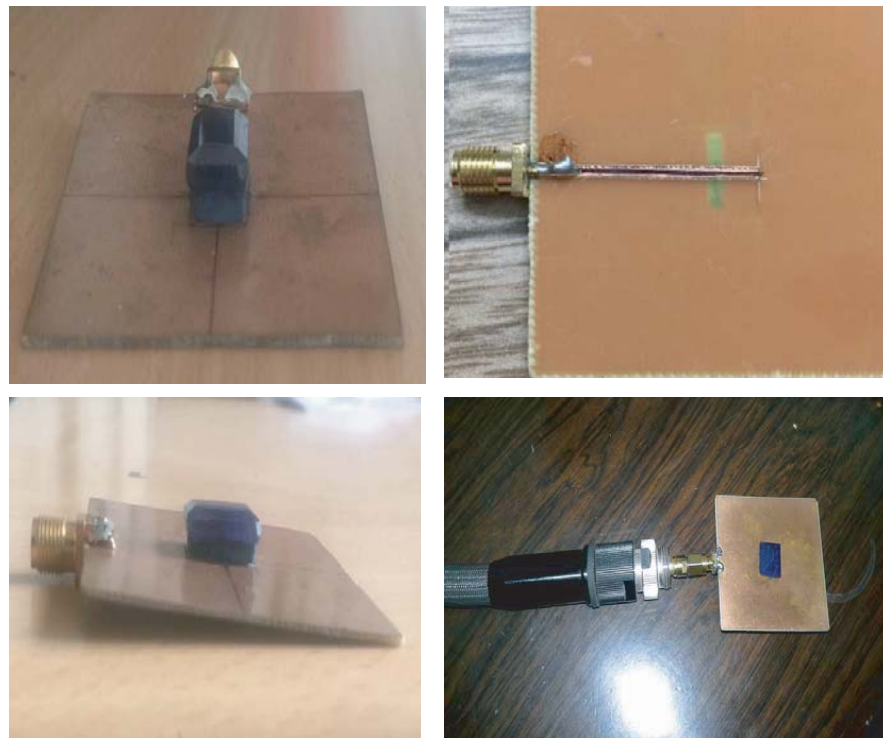
Figure 5. Photographs of the fabricated stacked antenna top view/back view/side views.
