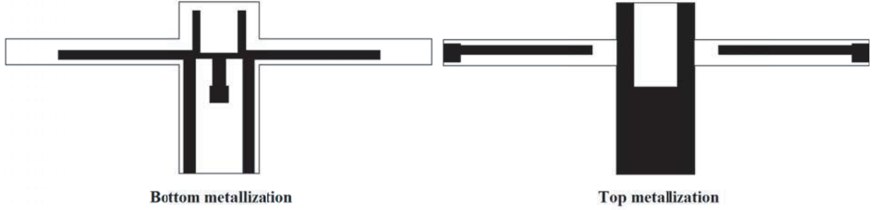
Figure 5. Top and bottom layouts of the SSL UWB BPF.
