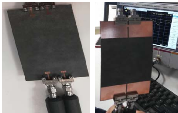
Figure 17. Photograph of introduced four element MIMO 5G antenna.
