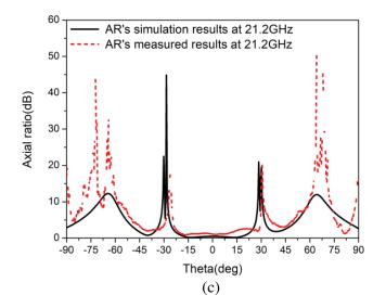
Figure 11. AR properties of the proposed antenna array.
