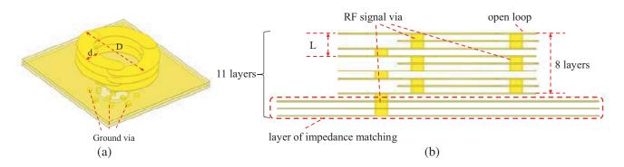
Figure 1. Structure of the proposed antenna element.
