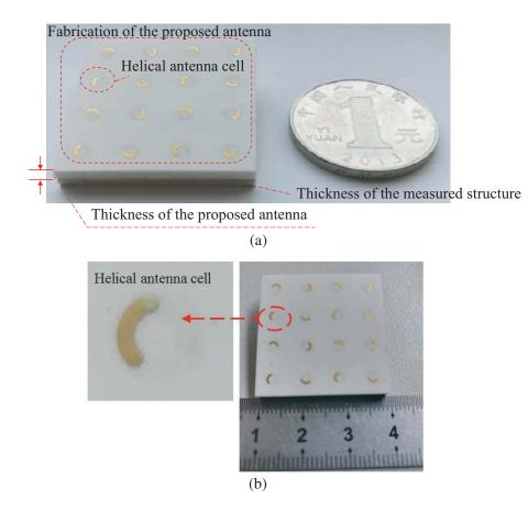
Figure 7. The fabricated RHCP antenna array.
