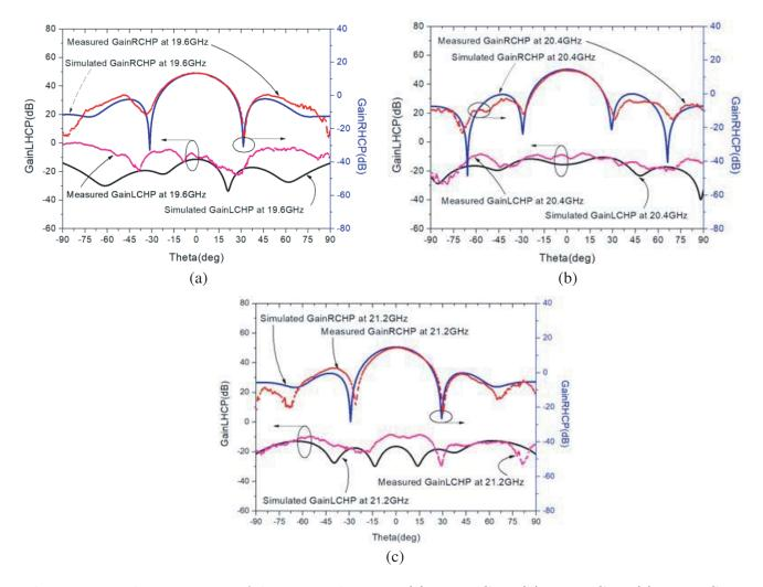
Figure 10. Radiation pattern of the proposed antenna (a) at 19.6 GHz, (b) at 20.4 GHz, (c) at 21.2 GHz.
