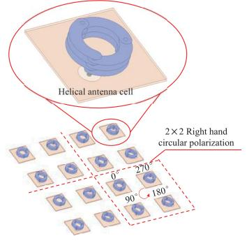
$4 \times 4$  helical antenna array
