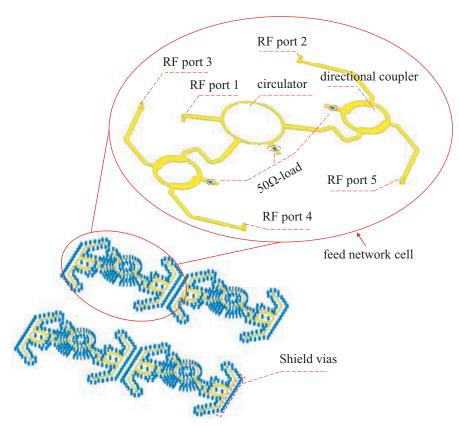
Figure 4. Structure of the proposed feeding network.
