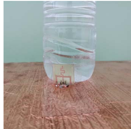
Figure 8. Impedance measurement by a baffle board method.
