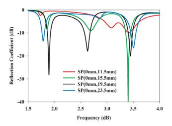
**Figure 4.** Parametric analysis of position of short element.
