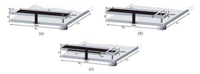
**Figure 1.** (a) Direct fed fundamental structure of PIFA, (b) capacitive fed PIFA antenna, (c) proposed triple band PIFA.
