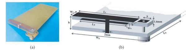
Figure 8. (a) Fabricated PIFA, (b) geometry of the proposed PIFA. The optimised design parameters are  $L_t = 35 \text{ mm}$ ,  $W_t = 5 \text{ mm}$ , s = 4 mm,  $L_b = 25 \text{ mm}$ ,  $W_b = 4 \text{ mm}$ , g = 0.5 mm, h = 6 mm,  $L_g = 10 \text{ mm}$ ,  $W_q = 40 \text{ mm}$ .
