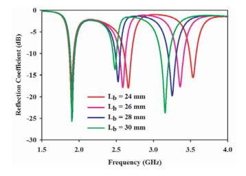
**Figure 7.** Parametric analysis of length of bottom radiating element,  $L_b$ .
