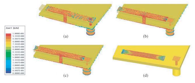
**Figure 3.** Surface current distribution, (a) fundamental PIFA, (b) first resonance of proposed PIFA, (c) second resonance of the proposed PIFA, (d) third resonance of the proposed PIFA.
