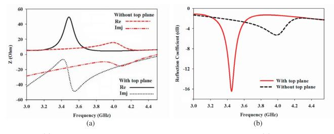
**Figure 6.** (a) Variation of impedance matching with the presence of top plane, (b) reflection coefficient of third resonance with and without top plane.
