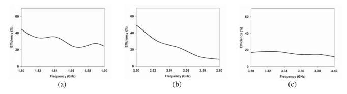
Figure 12. Measured efficiency response of the proposed antenna at (a) GSM 1800, (b) LTE 2500, (c) WiMax.
