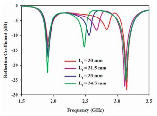
Figure 5. Parametric analysis of length of top radiating element,  $L_t$ .
