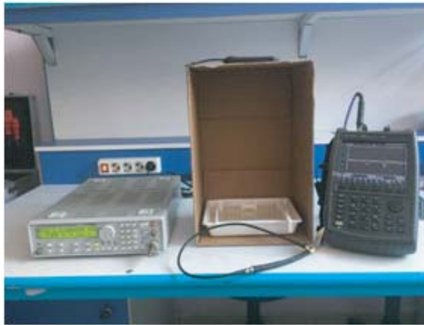
Figure 8. The experimental setup for infrared thermography. a) Signal generator, c) vector network analyzer, e) inside of the dark box, b) infrared camera, d) semi-liquid gel phantom and eyewear glasses.
