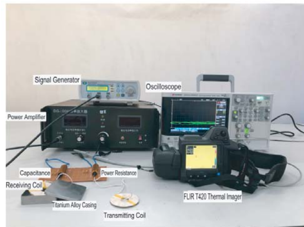
Figure 9. Experimental platform for the implantable medical device radio energy transmission system.
