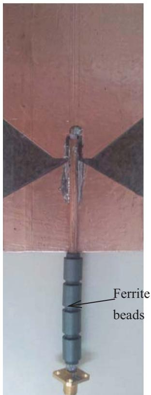
**Figure 7.** Photograph of proposed printed dipole antenna.
