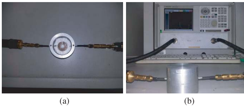
Figure 4. (a) Top view of resonator without lid. (b) Experimental setup.
