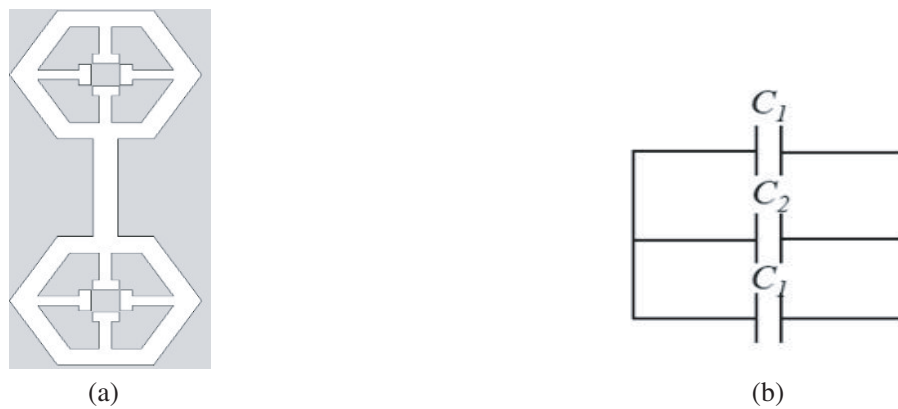
Figure 1. (a) The proposed model of DGS; (b) equivalent circuit (dark colour for metal and light colour for substrate).
