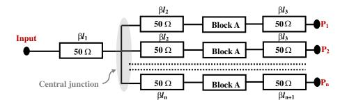
Figure 5. Simplified model of SPnT switch where Block A is defined in Figure 3(b).
