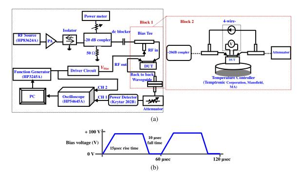
Figure 7. (a) Test set up and (b) bias waveform for reliability characterization.
