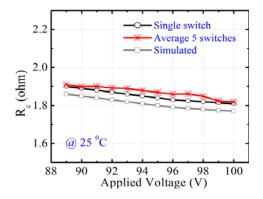
Figure 8. Measured contact resistance versus applied voltage for single lateral MEMS switch.
