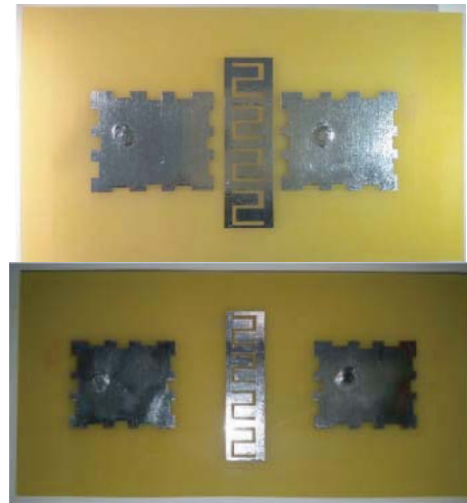
Figure 12. Prototypes of cut side microstrip patches with EBG structure at two different distances ( \lambda_0 , \lambda_0/3 ).
