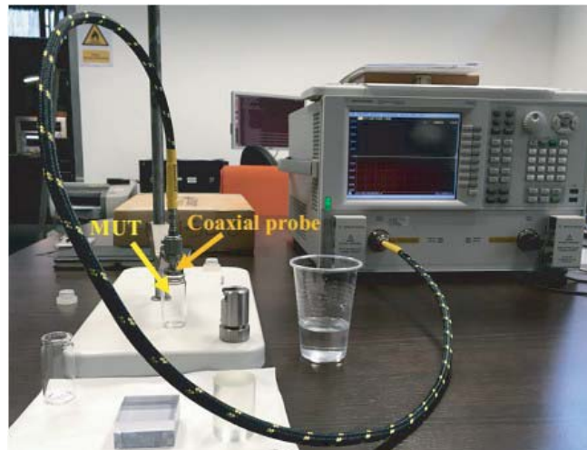
Figure 12. Equivalent dielectric permittivity measurement set-up.
