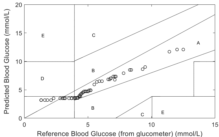
Figure 14. All the predicted blood glucose data is located in Zone A of Clarke Error Grid.
