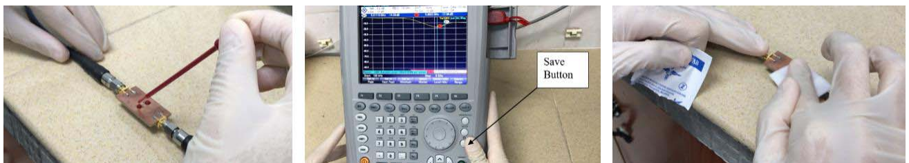
Figure 9. Collecting notch frequency shifting by using VNA.
