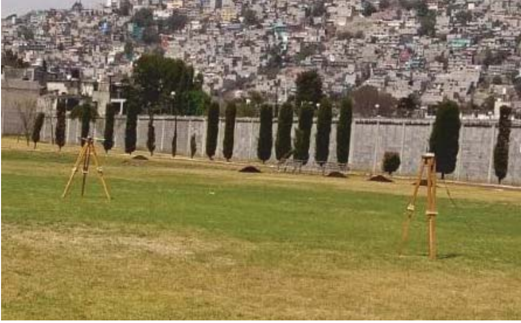
Figure 3. Disposition of radios for a single 50 m straight line, drone (left), GST (right).
