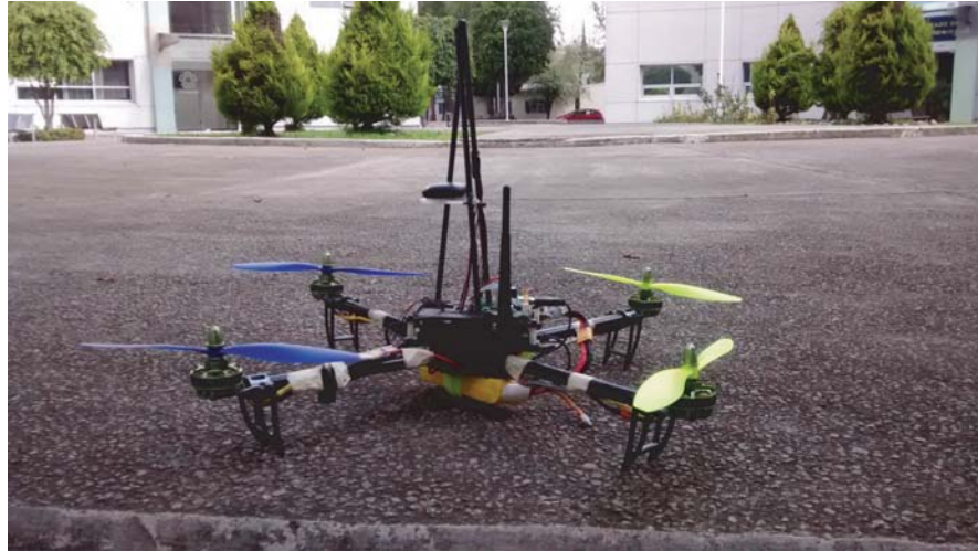
Figure 2. Drone with a 2.4 GHz radio onboard.
