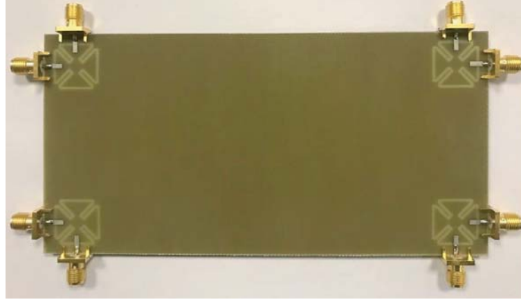
Figure 12. Fabricated smartphone antenna PCB.
