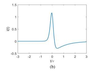
**Figure 2.** The charge and current pulses based on the approximating finite-rise time source functions (51) and (52). (a) Charge pulse. (b) Current pulse.
