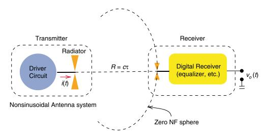
**Figure 1.** A general near-field communication system utilizing a nonsinusoidal antenna (NSA) transmitter. The NSA itself is composed of a driver circuit and a radiator. In contrast to mainstream sinusoidal antennas, the driver circuit, which produces the specialized nonsinusoidal signal i(t), must be designed *jointly* with the radiator itself. The Receiver is composed of a receive probe connected to digital receiver that includes an equalizer and other signal processing blocks.
