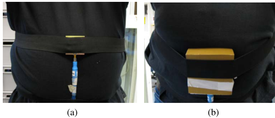
Figure 18. On-body measurement setup using the proposed UWB antenna (a) without and (b) with cavity.
