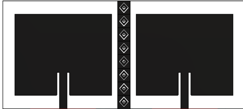
Figure 10. 2 \times 2 MIMO antenna with the 2nd iteration fractal EBG.
