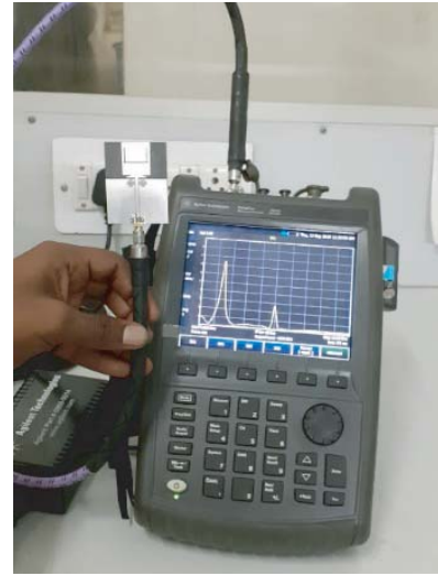
Figure 8. Antenna measurement using VNA.
