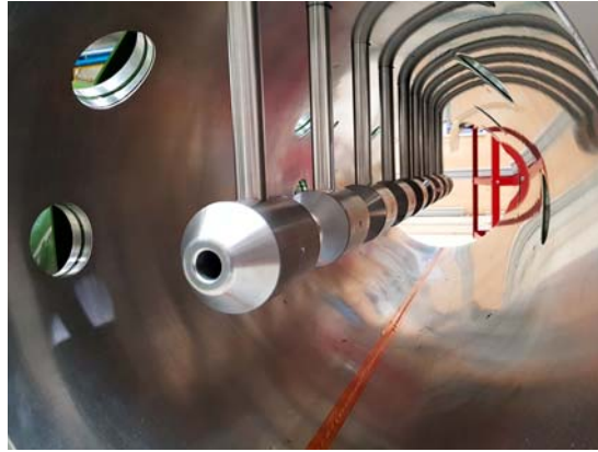
Figure 1. Internal view of a DTL cold model for RF tests. The drift tubes (central elements) are connected to the tank outer wall through physical metallic supports called stems.
