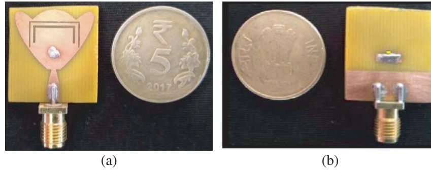
Figure 5. Prototype of the proposed antenna. (a) Top view and (b) bottom view.
