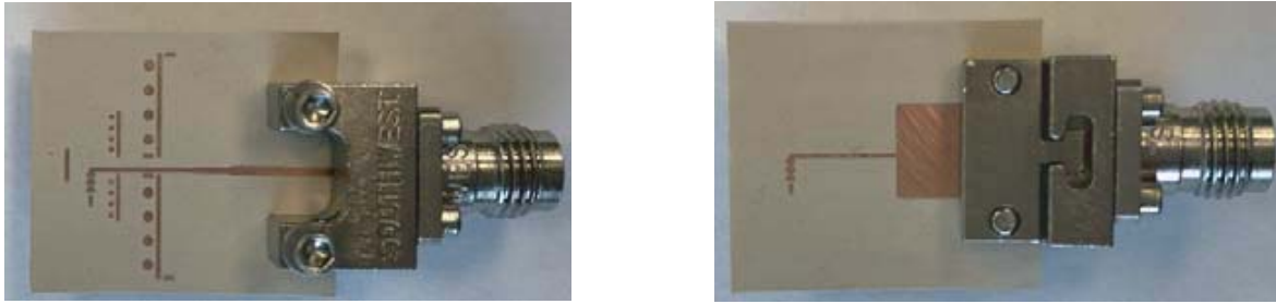
Figure 10. Photograph of the fabricated prototype of the dual-band 28/38 GHz Yagi-Uda proposed for MIMO antenna systems of 5G mobile handsets.
