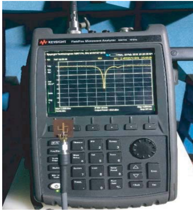
Figure 8. Photograph of measuring the reflection coefficient with Network analyser.
