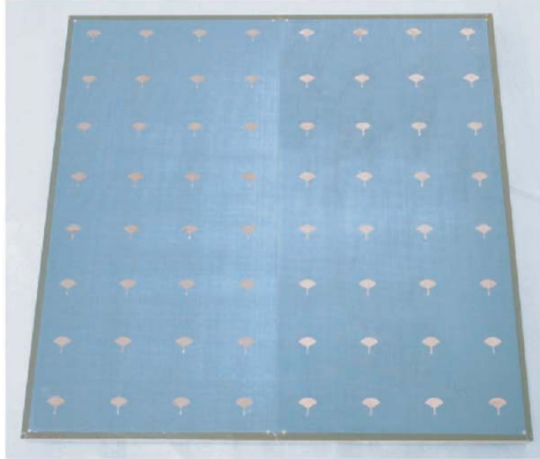
Figure 3. Photo of the prototype of 64-element antenna array. The profile of the array antenna is about 19.3\text{ mm} .
