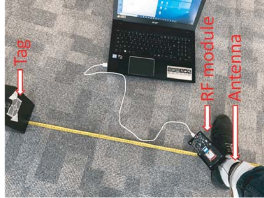
Figure 17. Photography of RFID functional reading distance test of the proposed antenna when it is placed on the human ankle.
