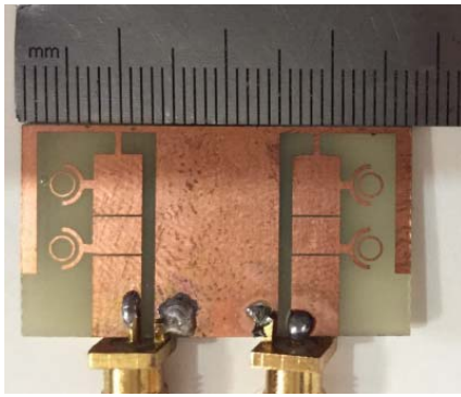
Figure 5. Photograph of the fabricated antenna.
