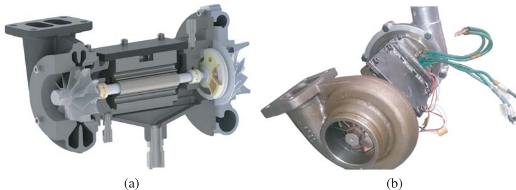
Figure 1. High-speed micro-CAES system: (a) three-dimensional model; and (b) assembled micro-CAES prototype [10].
