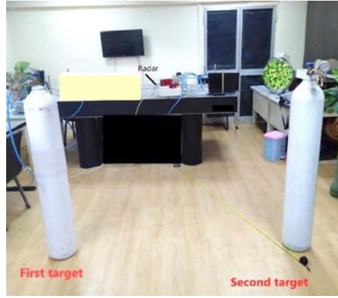
Figure 19. Experimental setup of the radar system to detect N = 2 metallic targets from two different directions -20^\circ and 43^\circ at M = 4 elements and K = 256 samples.
