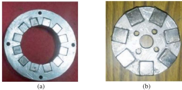
**Figure 12.** Cubical shaped magnets on a (a) Stator. (b) Rotor of a RMD configuration [88].
