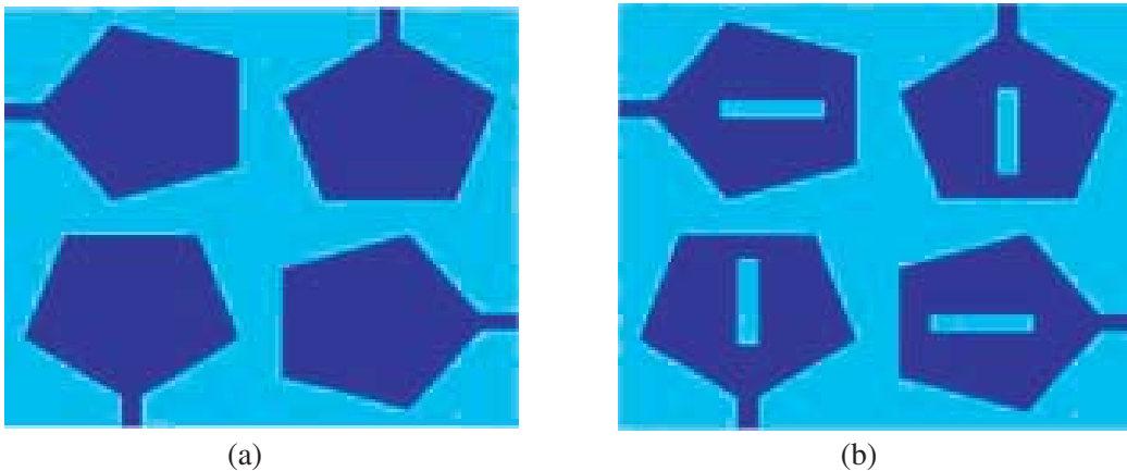
Figure 3. Configuration of the quad-port MIMO antenna. (a) Without rectangular patch slot. (b) With rectangular patch slot.
