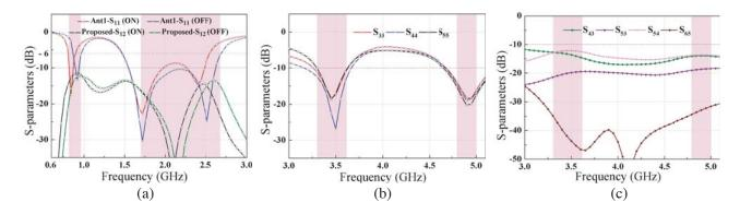
Figure 4. Simulated S-parameters of (a) 4G antenna elements, (b) and (c) 5G antenna elements.
