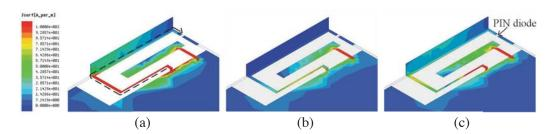
**Figure 3.** Surface current distribution when the PIN diode is in the OFF state: (a) 900 MHz, (b) 1700 MHz and (c) 2550 MHz.
