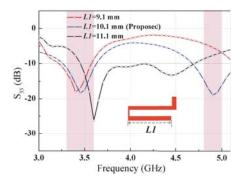
**Figure 5.** Simulated  $S_{33}$  of the Ant3 as a function of L1.
