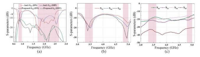
Figure 8. Measured S-parameters of (a) 4G antenna elements, (b) and (c) 5G antenna elements.
