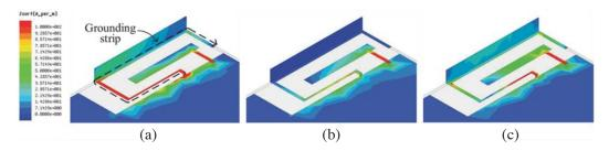
**Figure 2.** Surface current distribution when the PIN diode is in the ON state: (a) 850 MHz, (b) 1700 MHz and (c) 2400 MHz.
