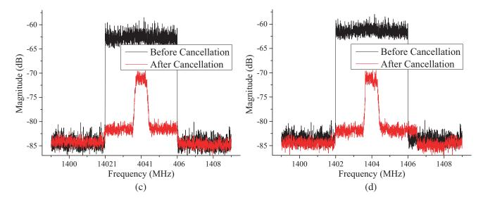
Figure 13. Spectrum of the signal before and after cancellation. (a) Interference suppression at  $-3^{\circ}$ . (b) Interference suppression at  $+3^{\circ}$ . (c) Interference suppression at  $-85^{\circ}$ . (d) Interference suppression at  $+85^{\circ}$ .
