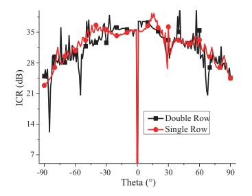
Figure 9. The ICR of two auxiliary antenna array layouts.
