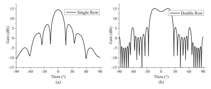
Figure 8. The pattern of two auxiliary antenna arrays. (a) Single row. (b) Double row.
