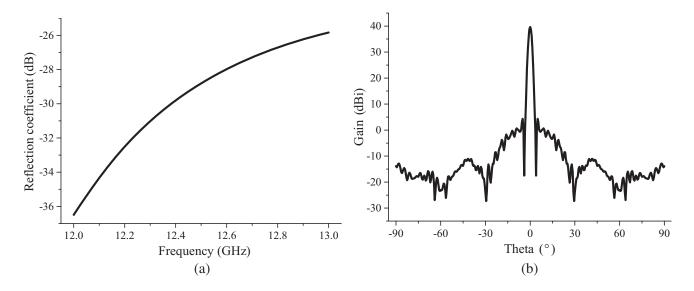
Figure 2. Simulated results of satellite antenna. (a) Reflection coefficient. (b) Radiation pattern.
