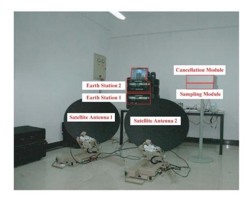
Figure 10. Satellite interference cancellation experiment system.
