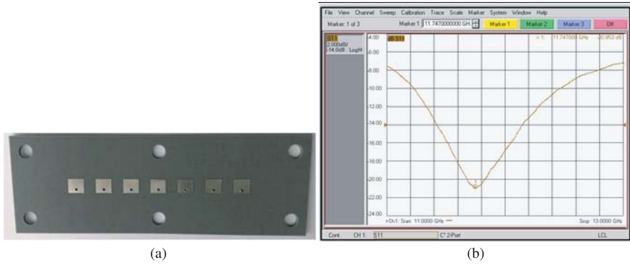
Figure 11. The fabricated and tested results of a 7-unit linear auxiliary antenna array. (a) Fabricated antenna. (b) Reflection coefficient.
