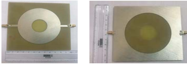
Figure 22. Top view and bottom view of fabricated proposed dual feed annular ring antenna.
