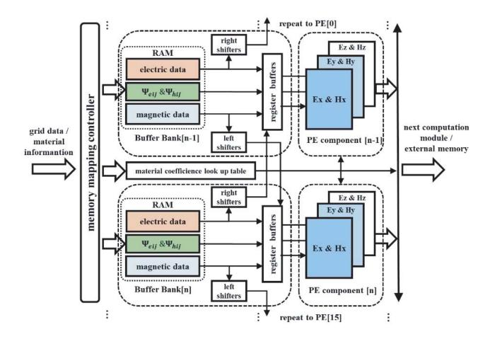
Figure 4. Framework of the chain PEs array. It consists of sixteen PEs. Shifters refer to several shift registers, which require one clock cycle to send a group with 32-bit data to other PEs.
