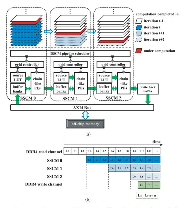
**Figure 6.** Schematic of the three-stage SSCM pipeline. (a) Dataflow of layers between SSCM stages. (b) Sequence diagram of data transfer among each SSCM stage and DDR4.
