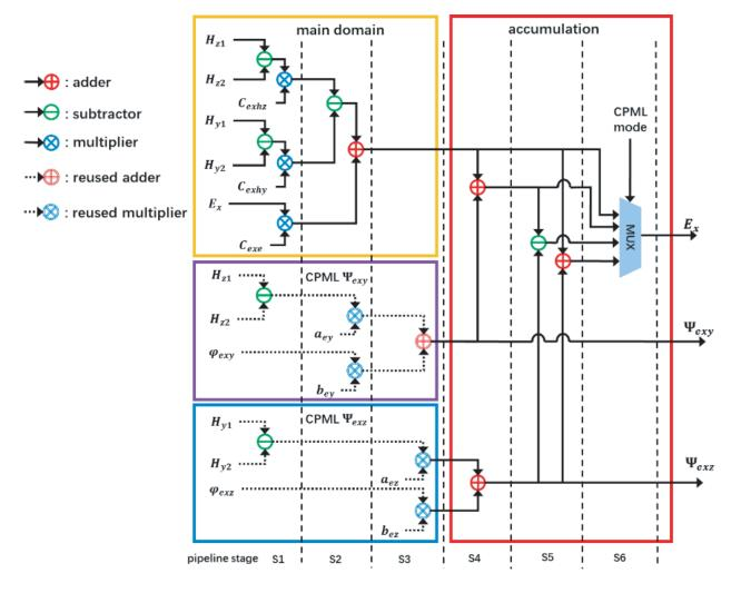
Figure 2. Schematic of the PE component module for processing  $E_x$ . The pipeline consists of six stages. The CPML mode signal in stage 6 is a 2-bit signal to denote four types of cell position occasions.
