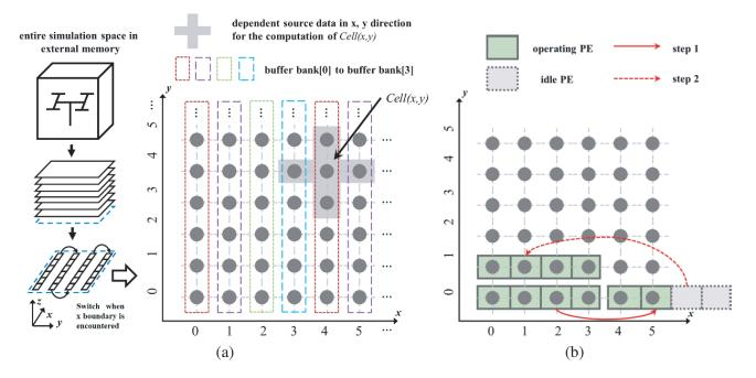
Figure 5. Memory mapping and corresponding computation mode of the chain PEs array taking a four-PE array as an example. (a) Data rearrangement method to transform a 3D grid to a 1D grid stream. (b) Cell scanning mode. The size of the layer is  $6 \times 6$ .
