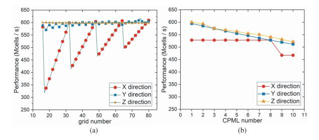
**Figure 8.** Performance test results for different grid sizes and CPML numbers in three directions. (a) Test results for different grid sizes. (b) Test results for different CPMLs numbers.
