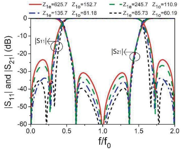
**Figure 5.** Responses of the proposed BSF with constant value of  $(1/Z_{1e} - 1/Z_{1o})$  ( $Z_2 = 159.7$ ,  $Z_3 = 78.8$ ,  $Z_4 = 138.7$ ).
