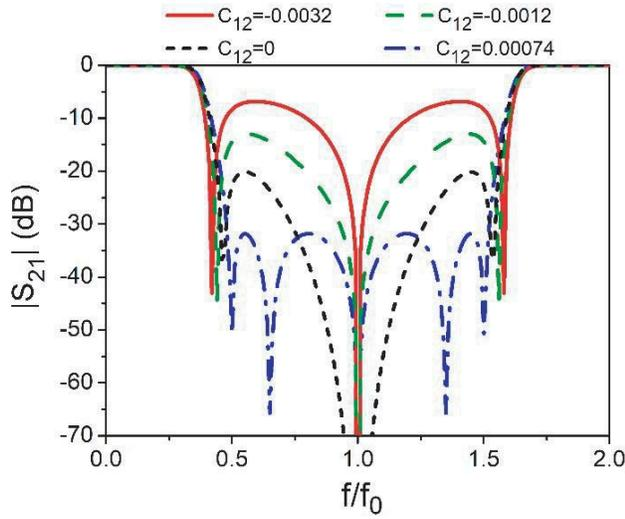
**Figure 4.** Responses of the proposed BSF with different  $C_{12}$  ( $C_1 = 1/68.77$ ,  $L_2 = 168.3$ ,  $C_3 = 1/30.4$ ,  $L_{12} = 408$ ).
