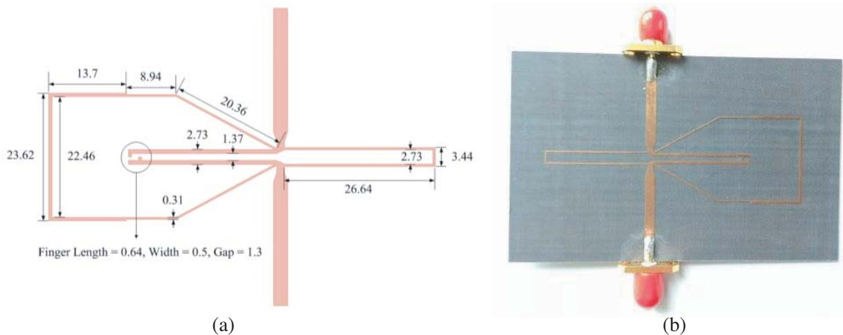
**Figure 8.** (a) Layout and (b) photograph of the example filter.
