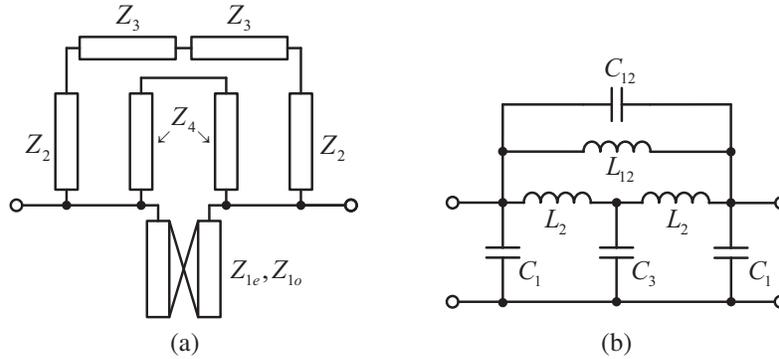
Figure 1. (a) Proposed BSF. (b) Lumped equivalent circuit.
