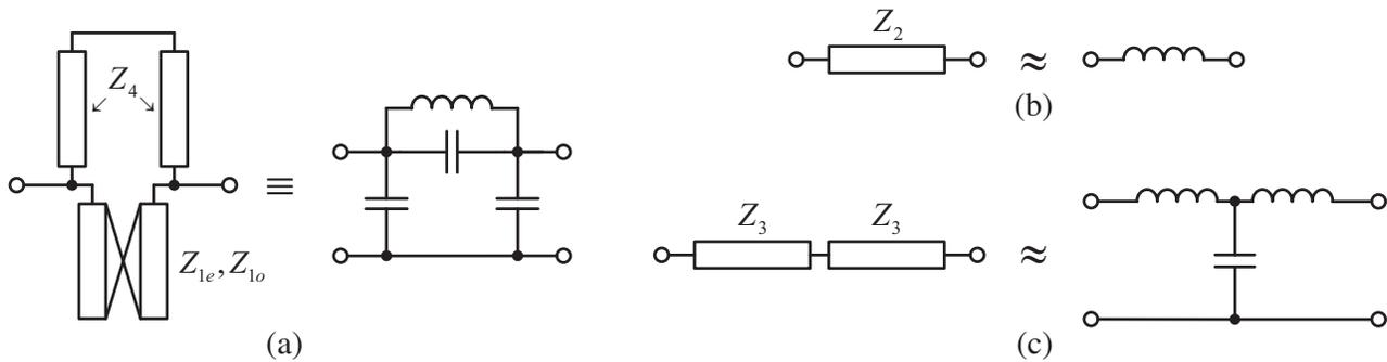
Figure 2. Detailed equivalences between the proposed BSF and its lumped equivalent circuit.
