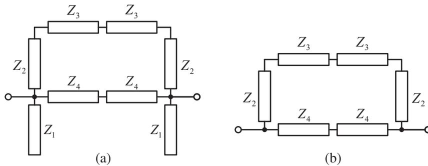
Figure 3. Ring BSFs (a) without cross coupling and (b) without shunt stubs.
