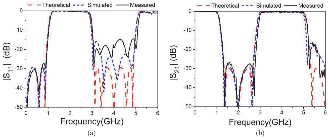
**Figure 7.** Theoretical, simulated and measured results of (a)  $S_{11}$  and (b)  $S_{21}$ .
