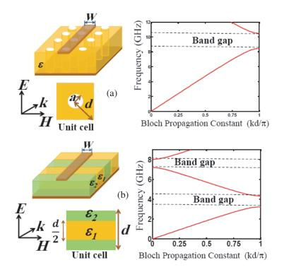
Figure 1. Photonic crystals used as substrates for microstrip structures (a) two dimensional photonic crystal designed with a background medium of  $\varepsilon = 4$  by carving cylinders of radius a = 0.25 cm, repeated with periodicity of d = 1 cm. (b) One dimensional photonic crystal consists of alternating materials of high and low dielectric constants of  $\varepsilon_1 = 2.3$  and  $\varepsilon_1 = 6.15$  with a periodicity 'd' of 2 cm.
