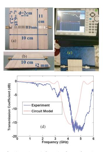
Figure 3. (a) Prototype of a 10 cm microstrip line printed on a photonic crystal substrate. The unit cell length is 2 cm and the dielectric layers consist of Rogers 5870 ( $\epsilon_r = 2.3$ ) and RO3006 ( $\epsilon_r = 6.15$ ). The effective relative permittivity of the substrate is 3.25. (b) Side view of the microstrip transmission line. (c) Measurement set-up with Anritsu MS2026 VNA. (d) Simulated and Measured transmission coefficient showing a bandgap between 4 GHz and 6 GHz.
