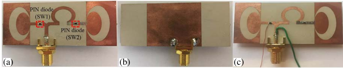
Figure 12. The fabricated antenna with PIN diodes; (a) front view, (b) back view and (c) biasing the PIN diode.
