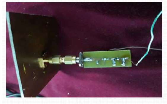
Figure 19. Prototype of the proposed rectenna element.
