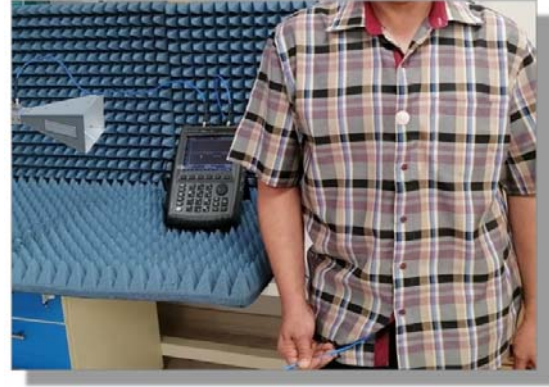
Figure 13. Experimental setup for measuring the radiation patterns of the conical-helix/monopole antenna when mounted on the human body using the VNA of the Agilent Field Fox N9918A.
