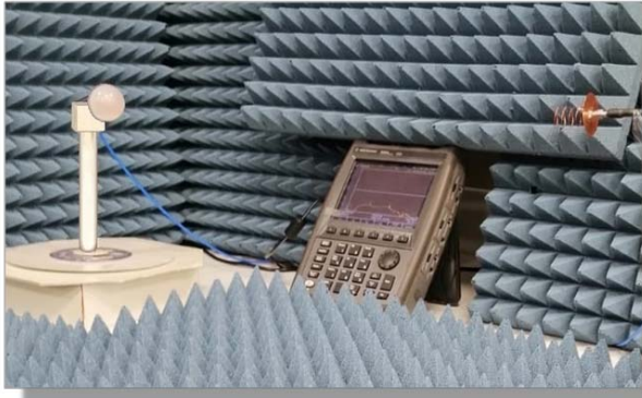
Figure 12. Experimental setup for measuring the radiation pattern of the proposed on-body conical-helix monopole antenna in free space using the VNA of the Agilent Field Fox N9918A.
