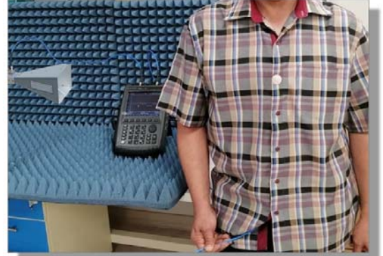
Figure 13. Experimental setup for measuring the radiation patterns of the conical-helix/monopole antenna when mounted on the human body using the VNA of the Agilent Field Fox N9918A.
