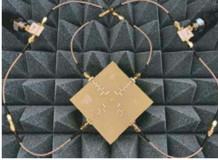
Figure 5. Measurement setup of the antenna system with wideband power dividers.
