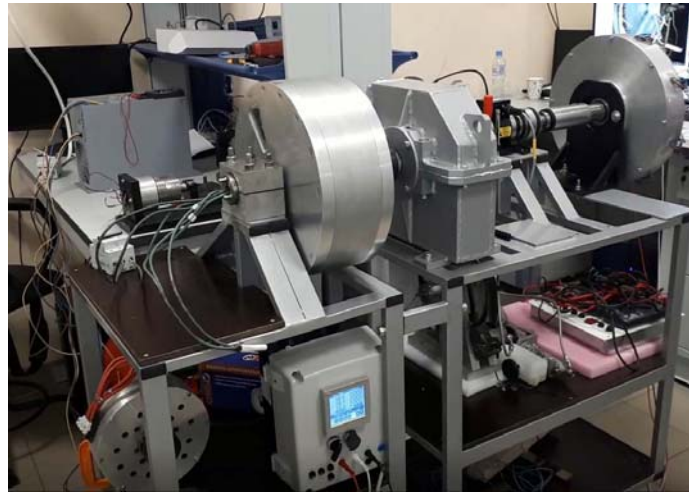
Figure 9. The stand for testing electrical machines (from left to right: traction motor; multiplier gearbox, Magtrol TM-311 torque sensor, axial flux machine; a digital multimeter is located on the middle shelf).
