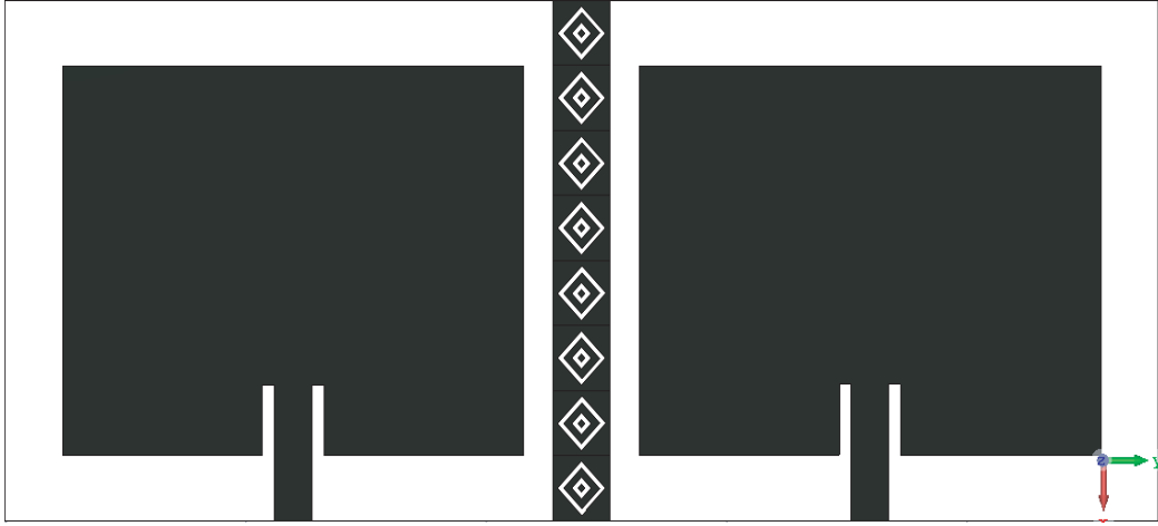
Figure 2. Antenna geometry of 2 \times 2 MIMO with DSFEBC structure.
