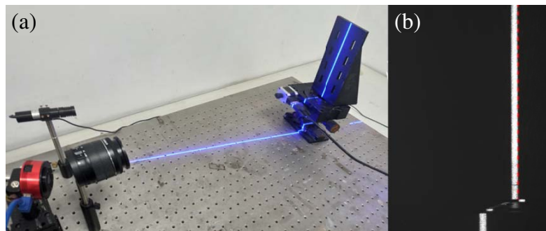
Figure 4. (a) Set-up with the Scheimpflug module and the rotary stage; (b) Image of the block.
