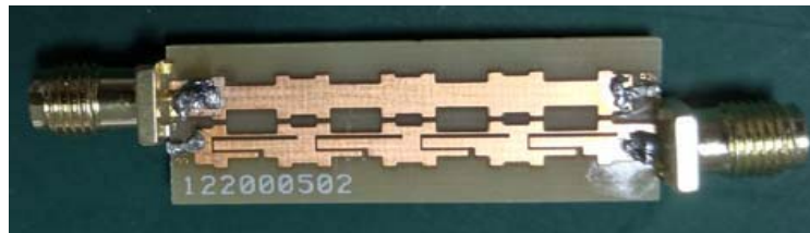
Figure 9. Actual production diagram of measuring far-end crosstalk S_{41} .
