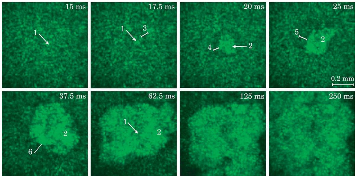
**Figure 7.** Frames of the high-speed imaging of nanoAl thin layer combustion obtained at the area of laser ignition using the scheme in Fig. 1(c). 1 — area of laser action; 2 — combustion products; 3–6 — combustion wave front.
