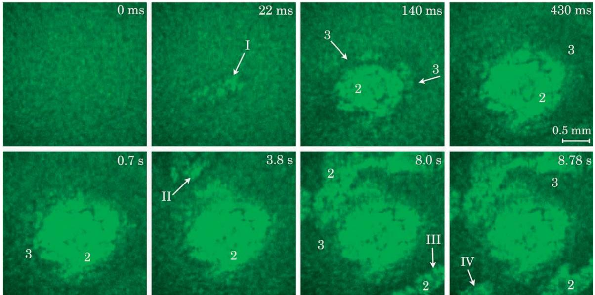
**Figure 5.** Frames of the high-speed imaging of nanoAl thin layer combustion obtained at the area of laser ignition using the scheme in Fig. 1(a). I — area of laser action; II–IV — areas corresponding to those marked in Fig. 3; 2 — combustion products/second combustion wave, 3 — first combustion wave.
