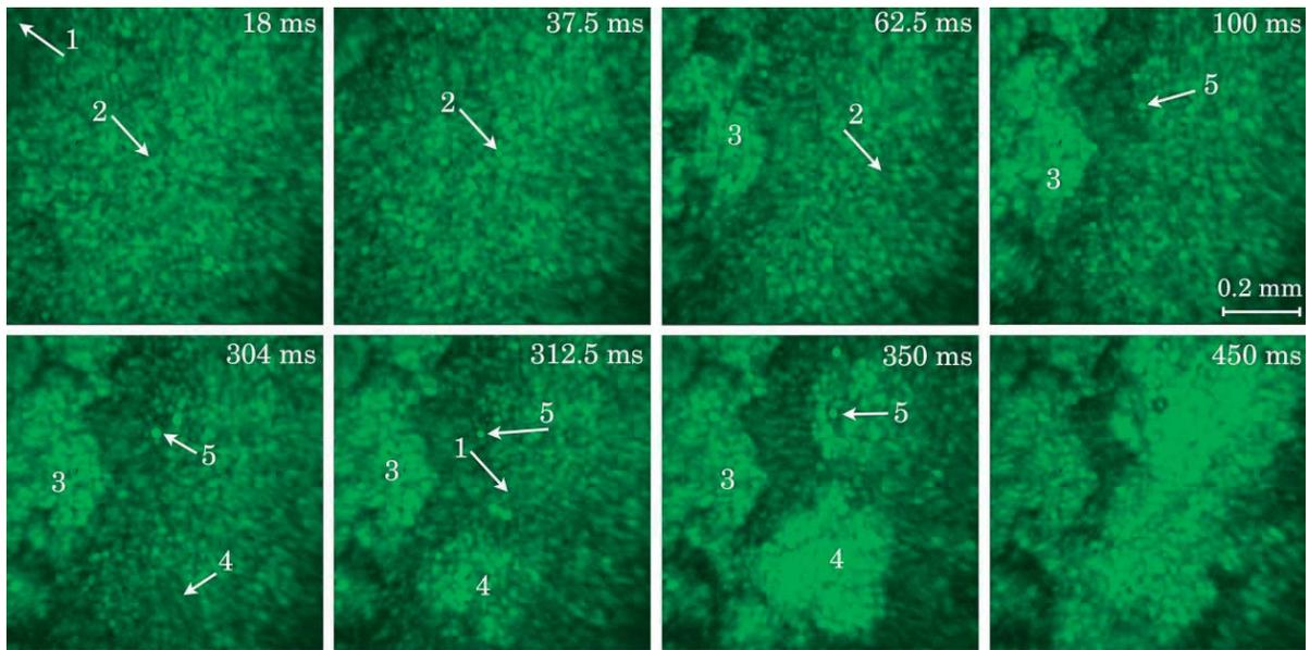
**Figure 6.** Frames of the high-speed imaging of nanoAl thin layer combustion obtained using the scheme in Fig. 1(b). 1 — area of laser action; 2 — front of the first combustion wave; 3, 4 — combustion products/second stage of combustion; 5 — liquid phase.
