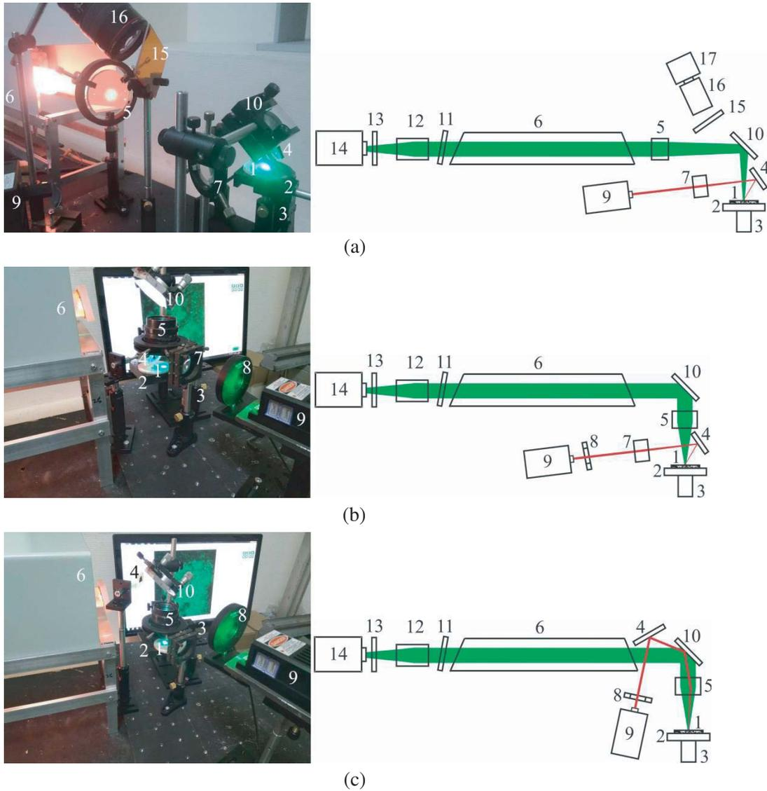
**Figure 1.** Schemes of the experimental setup. (a)–(c) Various implementations of laser monitors. 1 — nanopowder on a substrate; 2 — horizontal linear translator; 3 — vertical linear translator; 4, 10 — beam-deflecting mirrors; 5, 12, 16 — objective lenses; 6 — brightness amplifier; 7 — lens; 8 — mechanical shutter; 9 — igniting laser; 11 — neutral light filter; 13 — narrow-band filter  $510 \pm 5$  nm; 14 — high-speed camera; 15 — band-pass filter; 17 — USB-camera.
