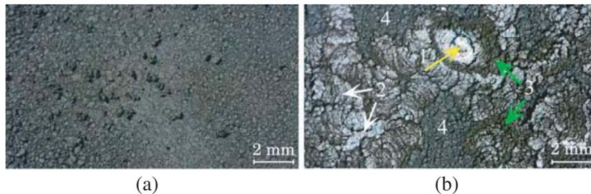
**Figure 4.** Typical view of the surface of the aluminum nanopowder layer. (a) Before combustion; (b) after burning out. 1 — area of laser action; 1, 2 — combustion products; 3 — unreacted aluminum; 4 — remains of the original aluminum nanopowder.
